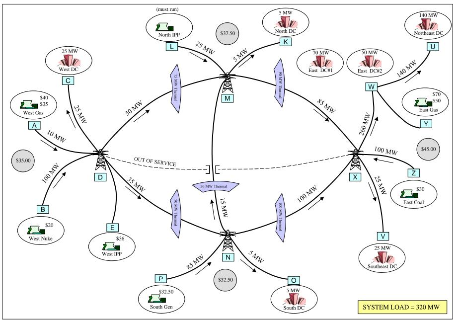
Generator Capacities: West Nuke, 100 MW; West Gas #1, 50 MW; West Gas #2, 50 MW; West IPP, 50 MW; North IPP, 35 MW; South Gen, 90 MW; East Gas #1, 50 MW; East Gas #2, 175 MW; East Coal, 100 MW
